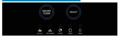
ON/OFF/CLEAN: Power switch button/Cleaning function button
